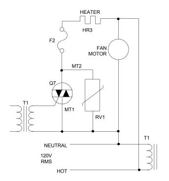
Figure 5-4. Case Heater Circuit
